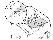
Fold out the extender, if necessary.
